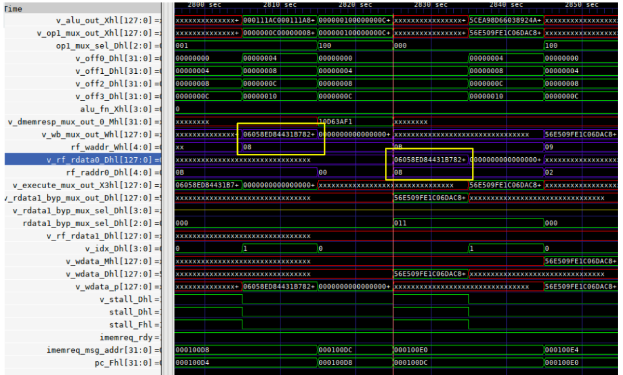
Figure 1: Waveform of vvadd benchmark showing v8 being written by load instruction and then later read by an add instruction
